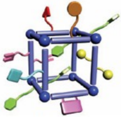
MTV-MOF-5 structure with eight different functionalities
